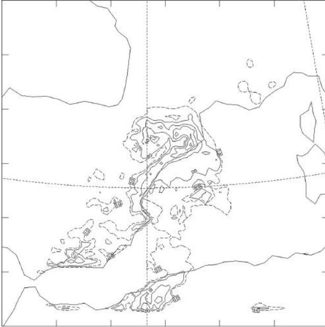
Figure 7.1 Forecast total precipitation from 06 UTC 10 October 1994 to 06 UTC 11 October 1994. Contour interval is 20 mm starting at 20 mm (continuous line). Dashed contour represents 10 mm. (Figure from Ramis et al. , 1998)
